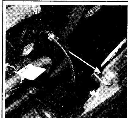
Fig. 30 Don't forget the bolt in inside the covers, at the top rear
