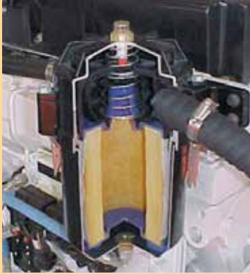
Cummins QSM11 marine engine with CCV cutaway
