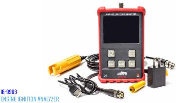
A handheld instrument designed from the ground up for the diagnosis and performance measurement of all types of spark ignition systems.
