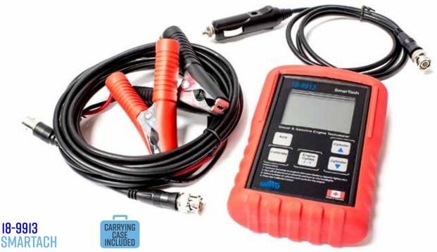
Designed for use on any engine equipped with an alternator, and only requires a simple connection to the electrical system (e.g. battery, alternator, cigarette lighter connector) to measure engine RPM. Taking advantage of the ripples generated by the alternator, SMARTACH automatically calculates the relationship between the speed of the engine and the alternator ripples, and uses them to measure RPM on any piston engine regardless of its ignition system (Diesel or gasoline).
