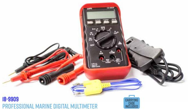
Offers full auto range features and functionality. Equipped with a 4 digit LCD display with analog bar graph it is capable of measuring AC/DC voltage up to 600 Volt and AC/DC current up to 10 A. Other functions includes tachometer for RPM measurement, dwell, temperature, resistance, frequency, fuel injection test, diode test, continuity check and overload protection.
